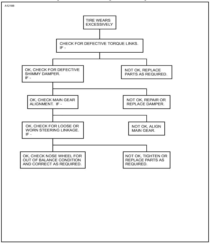
Figure 101: Sheet 1: Nose Landing Gear Troubleshooting Chart
