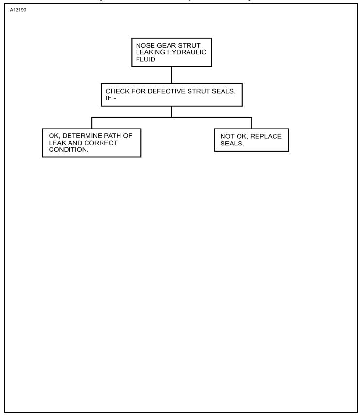
Figure 101: Sheet 3: Nose Landing Gear Troubleshooting Chart
