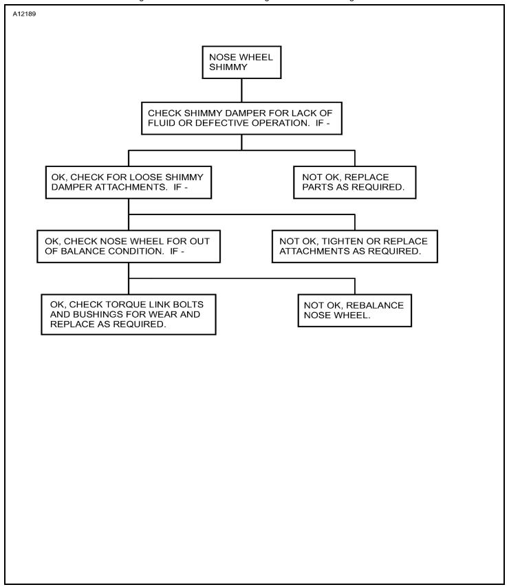
Figure 101: Sheet 2: Nose Landing Gear Troubleshooting Chart
